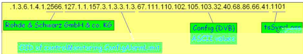
Fig. 21 OID formation process of a monitoring configuration variable
