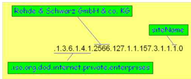
Fig. 16 OID formation process of simple variable
